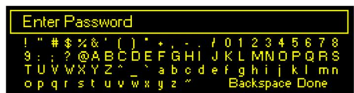
once more. The front panel will become fully accessible until the OLED timeout period has expired, which will then require the password to be entered again.
